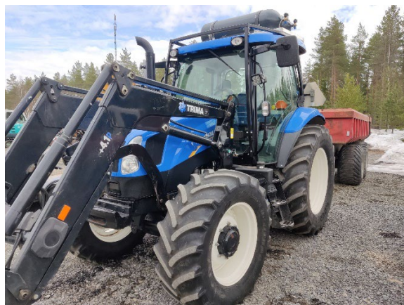
Figure 3 A tractor converted to operate on biogas. Photo Tapio Kyngäs
