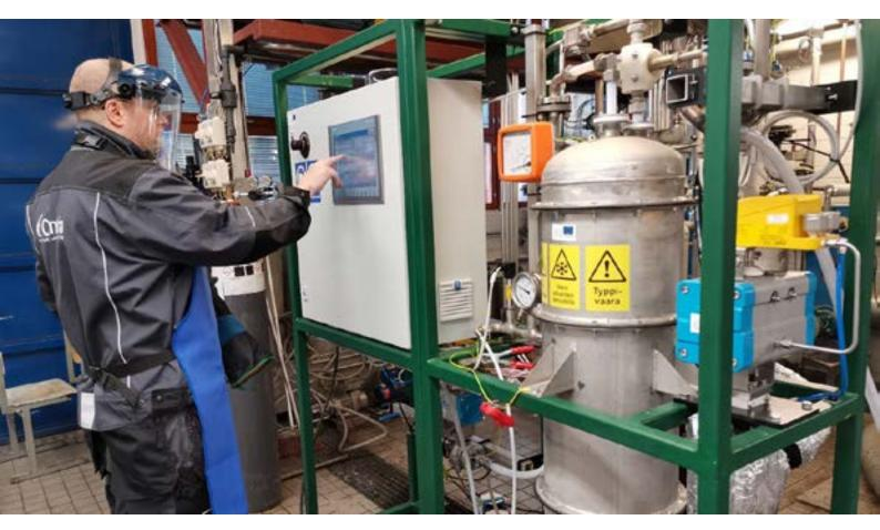
The aim of the project is to develop a new technology that will enable the smallscale liquefaction of biomethane in a cost-effective way. The liquefaction solution is based on the principle of cryogenic processing, which utilizes very low temperatures instead of high pressures to condense the gas.
